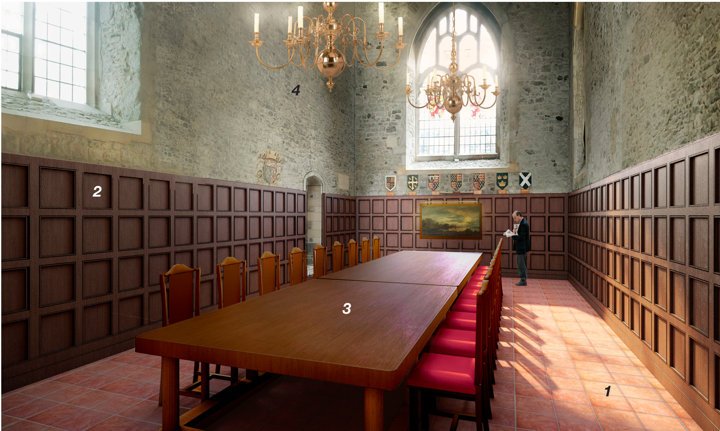
CGI image showing refurbished Chapel 1 New terracotta flooring replicates existing floor finish 2 Existing wall timber panelling made good with French Polish finish 3 Existing 'Mouseman' table retained 4 No 2 new chandeliers with LED lights to enhance lighting in the Chapel
